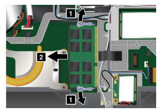
6. Find the notch on the contact edge side of the new memory module you are installing.
